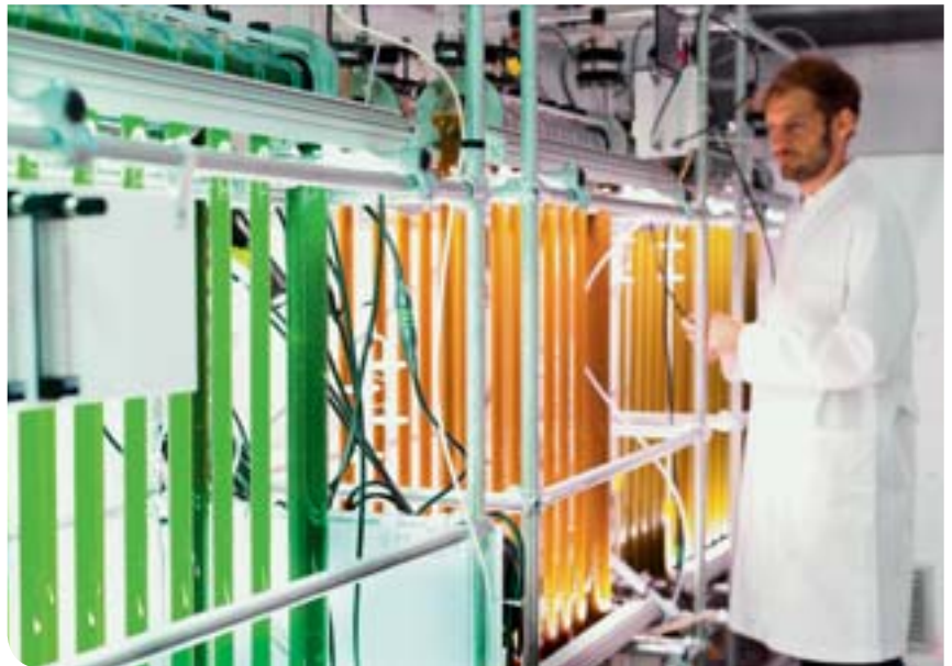
Mass cultures of snow algae in a linked-column photobioreactor system at Fraunhofer IBMT. Green snow algae in the active growth phase can be seen here on the left; on the right in the red, carotenoid-producing stress phase. © Tobias Marschner
